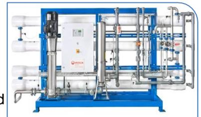
The system has been standardised and optimised in order to fulfil the essential demands of the relevant applications and minimise operating costs. With its high output, low-energy membranes it achieves a desalination rate of about 96 to 98% and at the same time, a water recovery of 100%.
